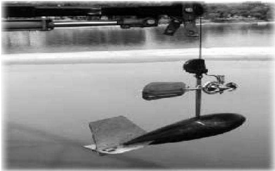
Fig. 11.3: A current meter inserted into the stream
